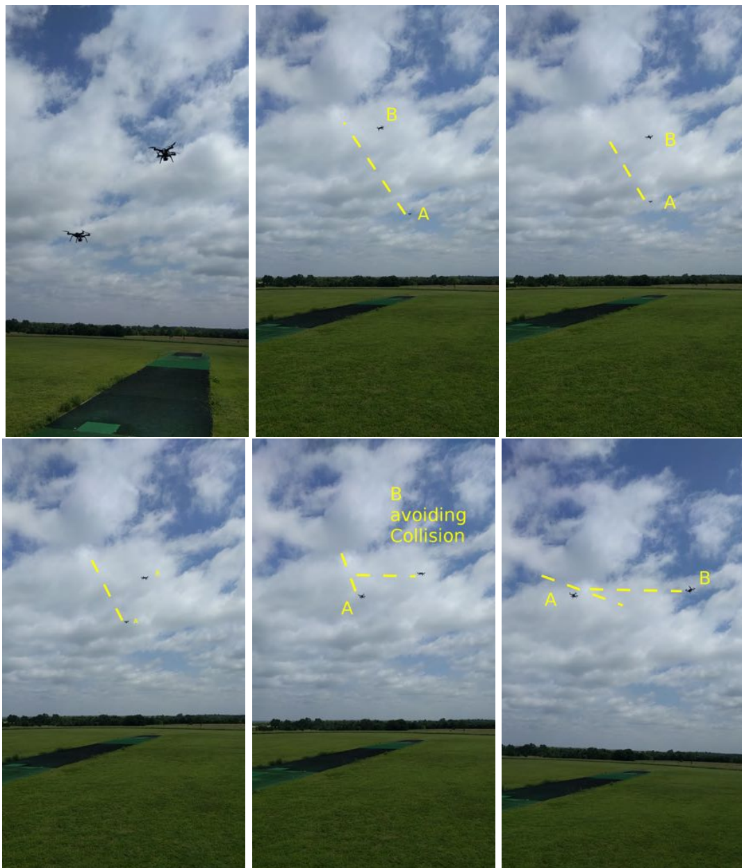
Figure 52: Experiment with two UAV robots A and B. (a) Robots take off. (b) Robots operating at safe distances from one another. (c) Human commands A to move toward B. (d) and (e) B moves to avoid collision with A. (f) A and B flying at safe distance again.
