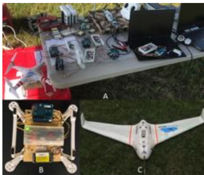
Figure 41: Illustration of the overall analytical setup for task 2-5 displaying (A) an overhead view of the ground station for the DJI P3 and the gas sensing packages; (B) an underside view of the instrument bed below the DJI P3 with a gas sensing package attached; and (C) a top view of the Skywalker X8 with the gas sensing packages secured in the instrument bed.
