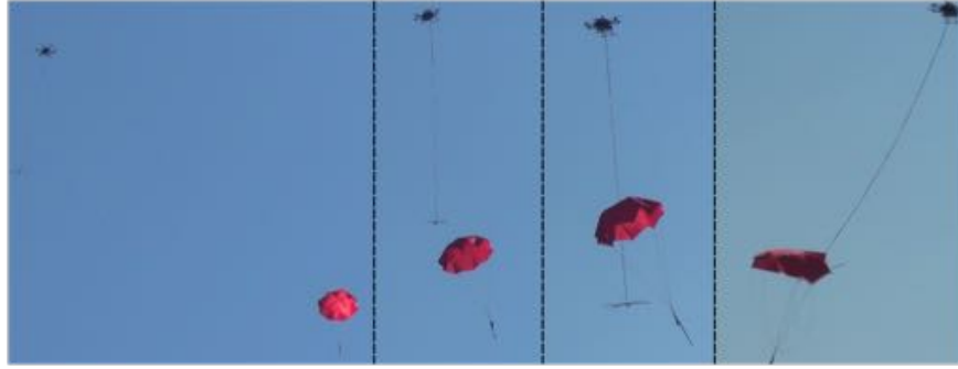
Figure 58: Four snapshots from a successful mission. The successive images show the UAS approaching the parachute from a distance, positioning itself before the maneuver, swooping towards the parachute, and finally trapping it in the hook.
