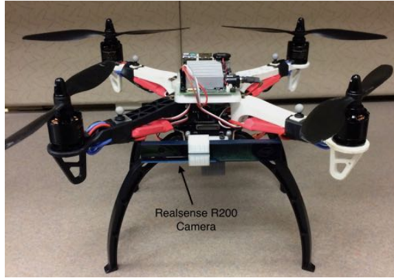
Figure 48: Front View of Fully Assembled Quadrotor. The Intel Realsense R200 is mounted to the front end.
